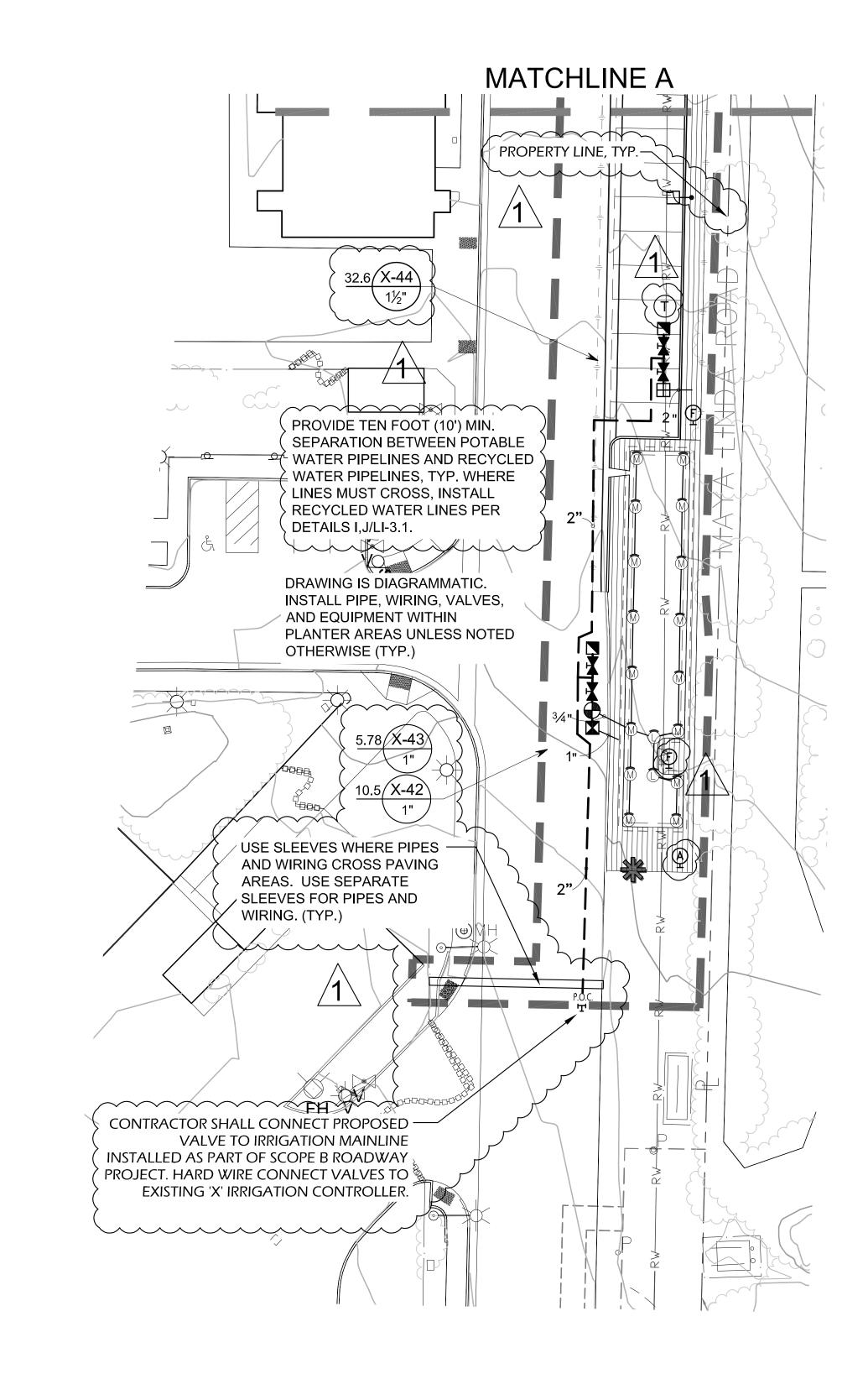
CITY OF SAN DIEGO WATER PRESSURE ZONES: 1) EXISTING RECYCLED WATER MAIN ON HILLERY DRIVE IS RECYCLED WATER PRESSURE ZONE No. 890 (ALL IRRIGATION SHOWN ON THESE PLANS IS RECYCLED WATER FROM THIS ZONE).
